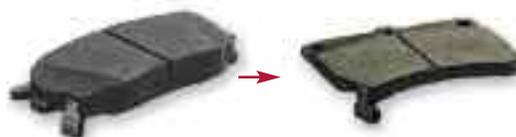
**Pad Wear Indicator:** When the pad reaches its minimum thickness, the indicator is against the disc and may make a squealing noise.
